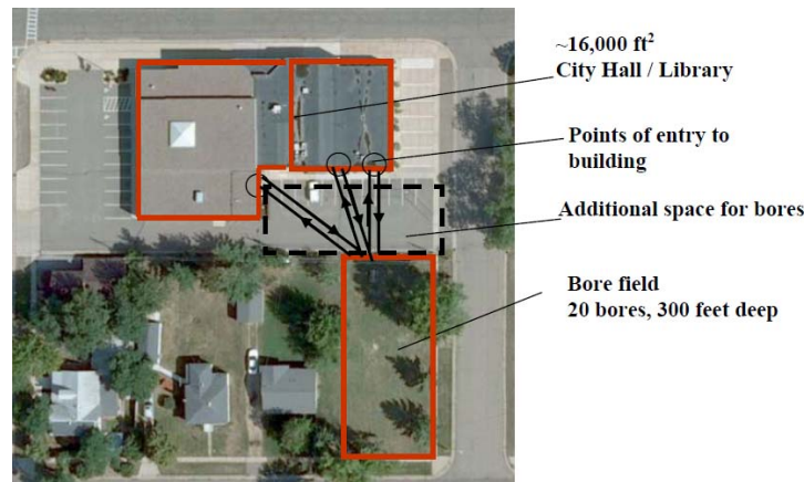
Figure 5. City Hall/Library Geothermal Bore Field Layout
